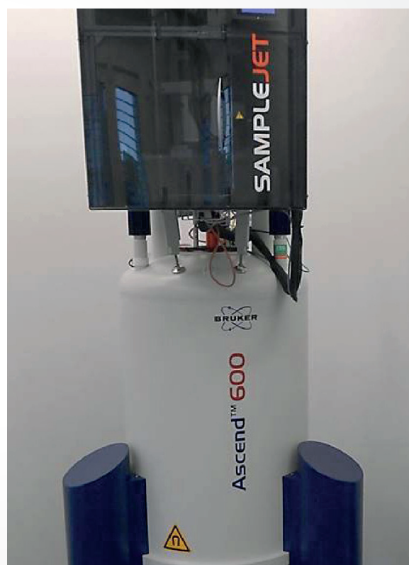
Figure 3: 600 MHz NMR spectrometer with SampleJet autosampler.
